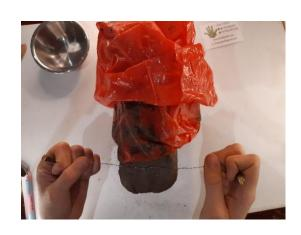
5. I made my own clay cutting wire using two twigs and some wire. I wound each end of the wire round the centre of each twig.
